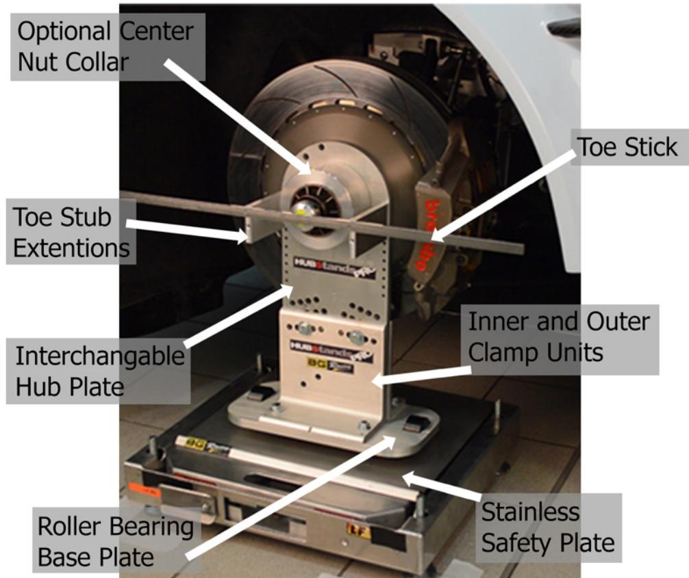
Making sure the HUBStands are centred on the scales and on the Safety Plates. Lower the car. Repeat on the other side. After the HUBStands are all on and the car lowered onto the scales, carefully rock the car side-to-side settling the suspension HUBStands are designed to easily roll laterally as the suspension settles, make sure you do not roll them to the edge of the Safety Plates. The actual amount of lateral "slip" will vary by individual vehicle and by hub. It may not even be noticeable.
