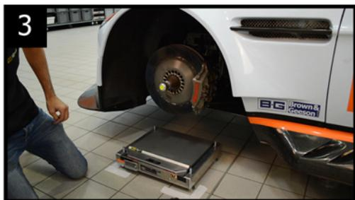
Jack the car one side at a time. Remove the wheels on the jacked up side (1, 2). Place your scale units in position (3) and attach the two HUBStands in the same manner you would a wheel, using all the lug nuts/bolts or centre lock collar and nut.
