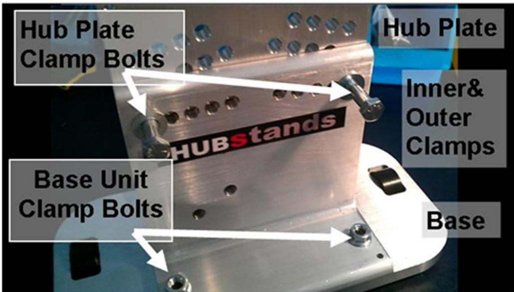
Adjust the Hub Plates in the other three HUBStands, relative to the height differences of each of the wheels. Make sure that both clamping bolts are in place on each HUBStand and that they are tightened to at least 30 lb/feet of torque.
