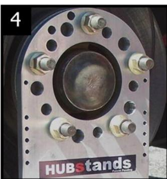
Tighten each nut/bolts or centre lock nut to at least 50lb./ft. of torque making sure they are flat against the face of the hub. Make sure both HUBStands labels on each unit are facing the outside of the vehicle (4, 5, 6).
